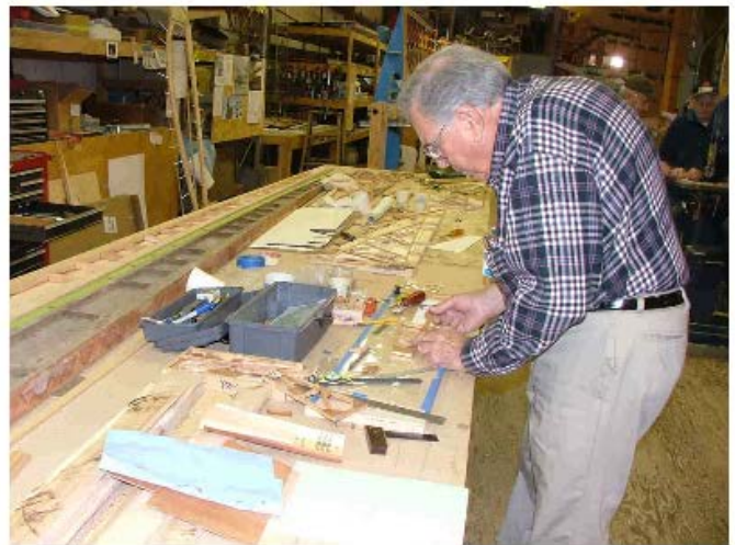
RCRC volunteers create wood spars and ribs from scratch for a Pratt-Read PR-G1 Glider used for Navy pilot training during WWII
