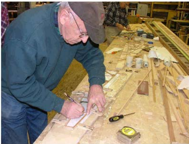
RCRC volunteers create wood spars and ribs from scratch for a Pratt-Read PR-G1 Glider used for Navy pilot training during WWII
